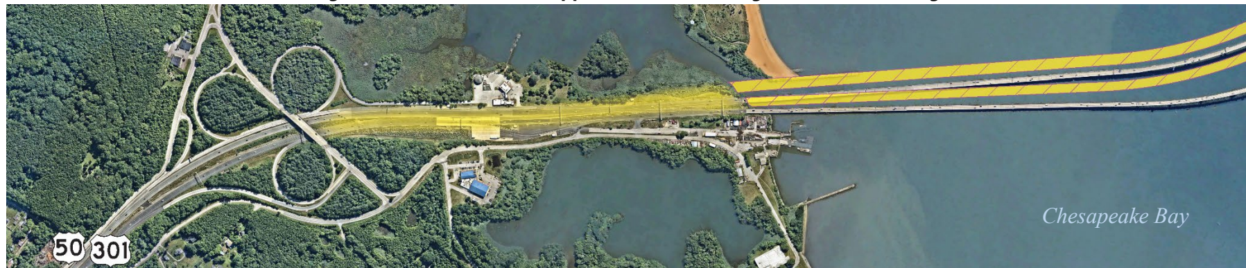
Figure 3.2. Western Shore Approach, Northern Alignment, 8-Lane Bridge
